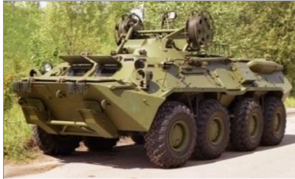
BREM-K (repair evacuation)
